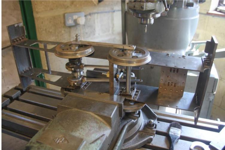
brackets, slide bars and crossheads. As well as these parts, we have found time to pin all four wheels to the axles by threading bored holes to take a 4mm grub screw. **(Photo above: The entire chassis mounted in the milling machine ready to drill 50:50 into each wheel and axle in order to pin them)**
