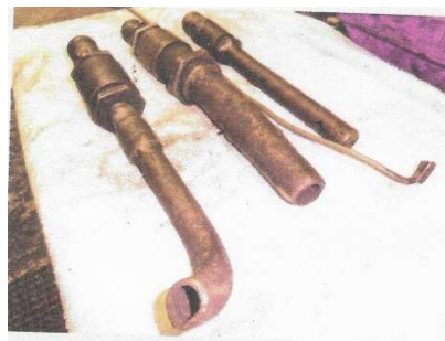
Boiler washout nozzles and rake for pulling out dislodged scale.
