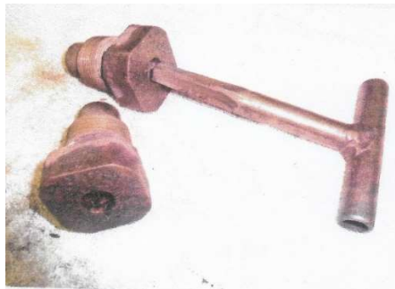
A tool for cleaning fusible plugs. This consists of a reamer section that cleared the char and scale to examine the lead core.
