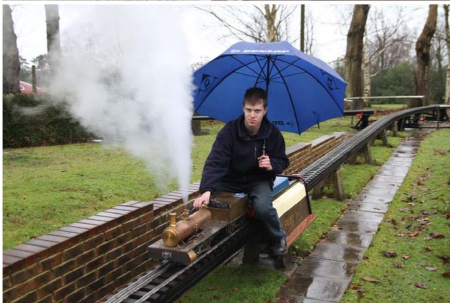
**Picture Top:** The first milestone was the completed boiler, successfully tested to 160psi
