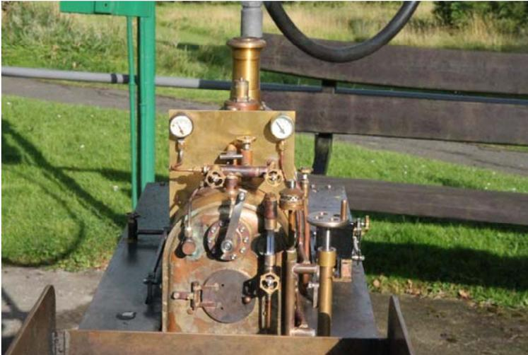
**(Pictures above and left: 'Dougal' standing on the steaming bays after its steam test. The exhaust seen in the first picture is from the vacuum ejector not the regulator leaking by!)**
