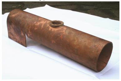
holes evenly around the circumference of both the bronze ring and flanged fitting in the back head. (Pictured above: My main boiler barrel complete with dome soldered in place and fire box sides opened out)
