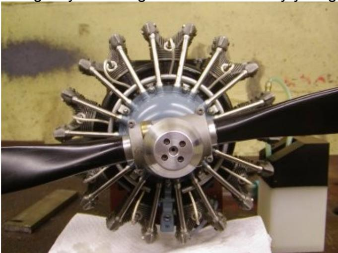
for many hours with no trouble, and stainless has proved perfectly satisfactory in this little "Wasp". The valve guides and valve seats (or valve cages) are one-piece jobs and had to be hollowed out so some cutters were made for machining. I had no phosphor bronze at the time, but found some beryllium copper of a convenient size on the shelf. This has proved to
